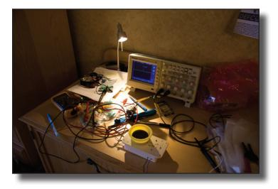
When we connected the Geiger counter up to the oscilloscope, the pulses registered as 80 volts in magnitude. After staring at the display for a few long minutes, we realized that the 10x probes were improperly configured in the menus of the oscilloscope. Remember that part about understanding the characteristics of your test equipment and how those characteristics affect measurement is part of the process of design, build, and test?
