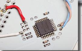
ohm resistor installed in the center position. We suspected that these were used to identify the type of badge to the processor.
