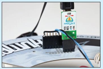
Seen above, the little red and blue arrows on the RX and TX lines made it easy to hook up correctly the first time.
